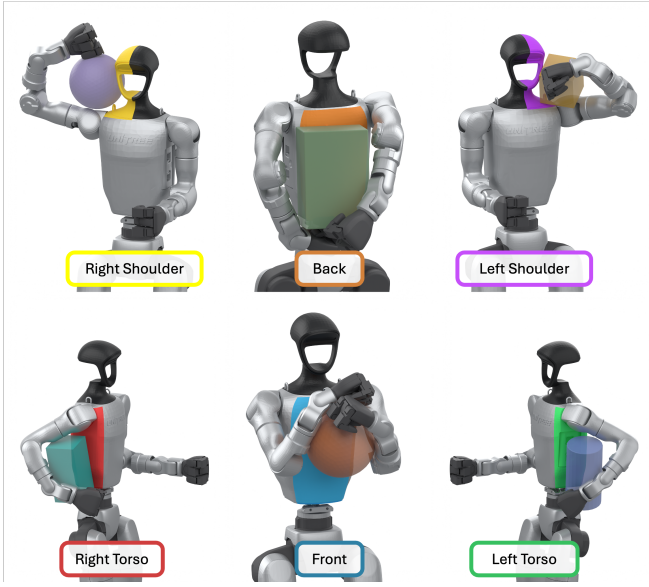
Fig. 7: Torso contact regions. One accepted grasp is shown per region, each on a different object.
